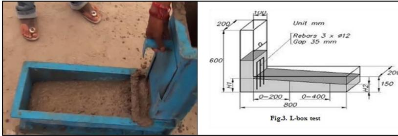
Figure 3 L-box test
