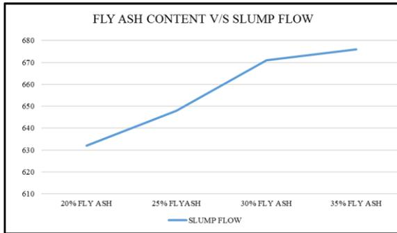
**Figure 5** Flow test results
