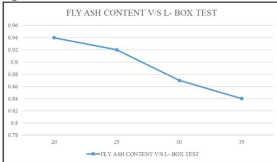
**Figure 7** L-box test results
