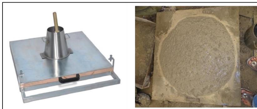
**Figure 2 Flow-cone and table test**
