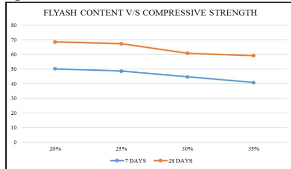
**Figure 8** Compressive strength test results
