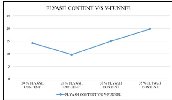
**Figure 6** Funnel test results
