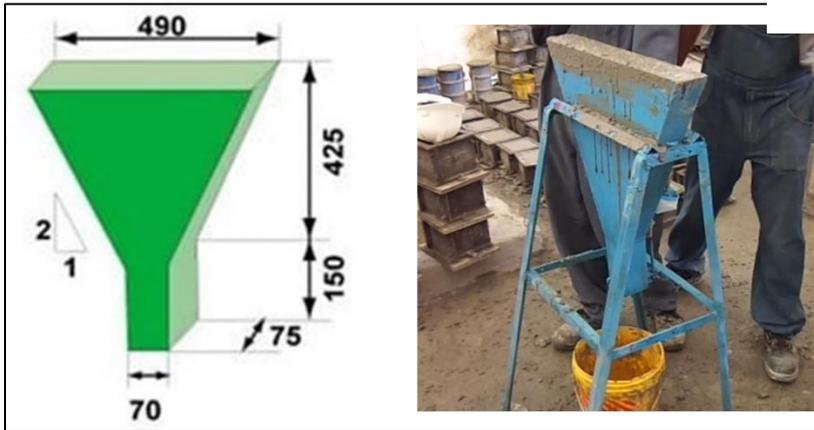
Figure 4 V-funnel test
