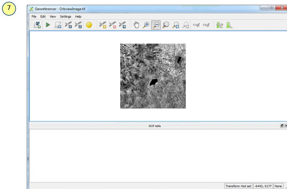
8. Next, identify and zoom into a feature that is easily identifiable on the image. Generally, features like road intersections or building corners are used. To zoom in to a feature
