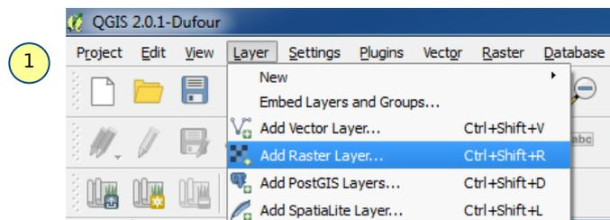
2. A window will pop up in which various files will be displayed. Click on the drop down menu below and select '**[GDAL] GeoTIFF**'. Navigate to the output folder of *IGET\_GIS\_003: Georeferencing* tutorial and select the georeferenced toposheet file ('*Toposheet\_WGS84\_georef.tif*') and click '**Open**'.
