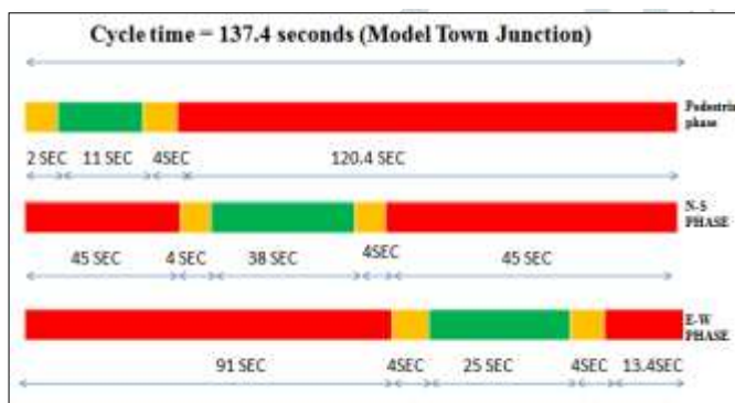
Figure 11 Signal phase cycle of Model Town Intersection
